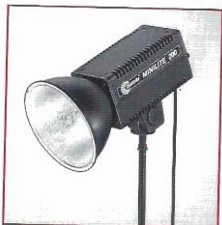
The standard reflector COMNOS for maximum light reflection. 16 cm diam.; 65°-angle of emission. Can be fitted with the diffuser PROSOF and the barn doors PROKLA for further light control.
